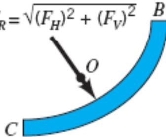
A diagram showing the resultant force  $F_R$  acting on the curved surface BC. The force is represented by a black arrow pointing towards a point O on the curve. The formula  $F_R = \sqrt{(F_H)^2 + (F_V)^2}$  is written above the diagram.
