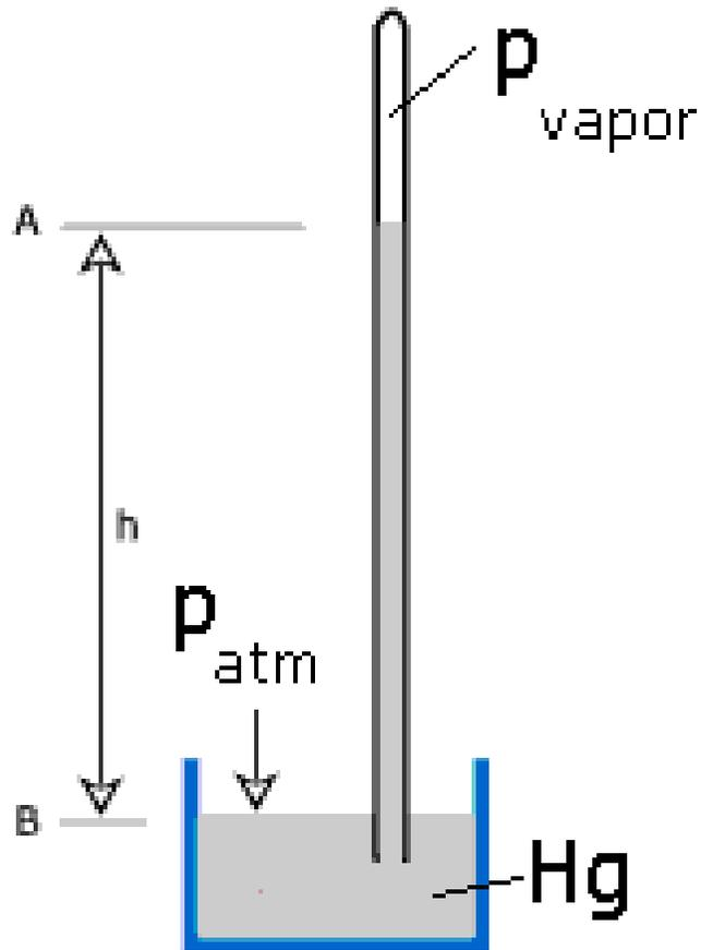
$$p_{\text{atm}} = \gamma_{\text{Hg}} h + p_{\text{vapor}}$$
